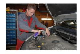
Electrical Connections are treated with 'Prolan' to prevent corrosion and moisture penetration.
